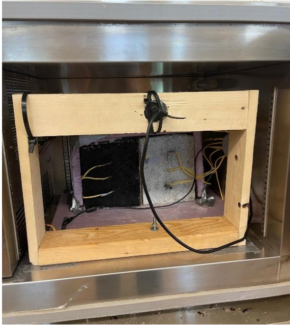
Fig. 15. Concrete samples are placed in the chamber with the thermocouples attached to the samples.
