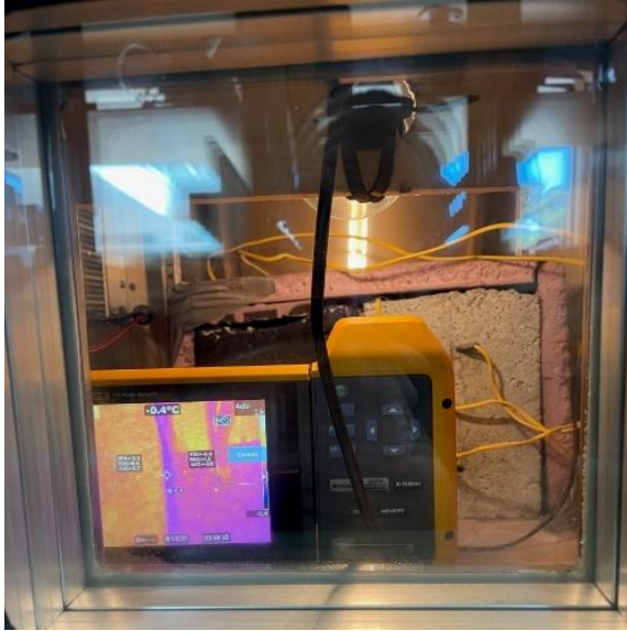
Fig. 14. An infrared camera is used in the chamber to calculate surface temperature.
