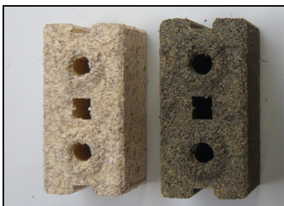
Fig. 5. Masonry samples produced using hemp hurd bast fibre in the form of interlocking blocks.
