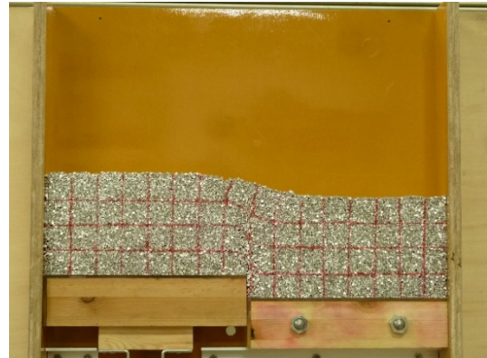
Fig. 11. Shallow aluminum model ground deformation after the vertical fault moved.
