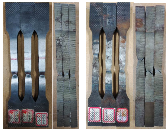
(a) 16 mm plate thickness (b) 20 mm plate thickness Fig. 2. Photographs of welded joint coupons with different thicknesses after failure.
